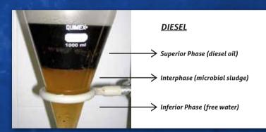
Fuel tanks accumulate water on a daily basis through the process of condensation (variation of the room temperature). Fuel absorbs water (hygroscopic effect) and its presence should be avoided as much as possible (periodic drainage) and constantly checked (water finding paste).
